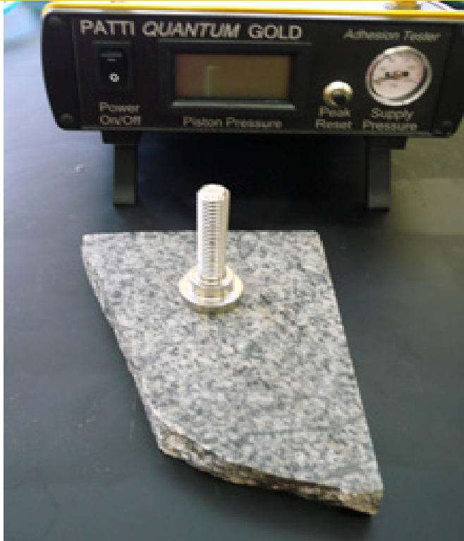
Aggregate Plate and stub. Digital display gives POTS.
