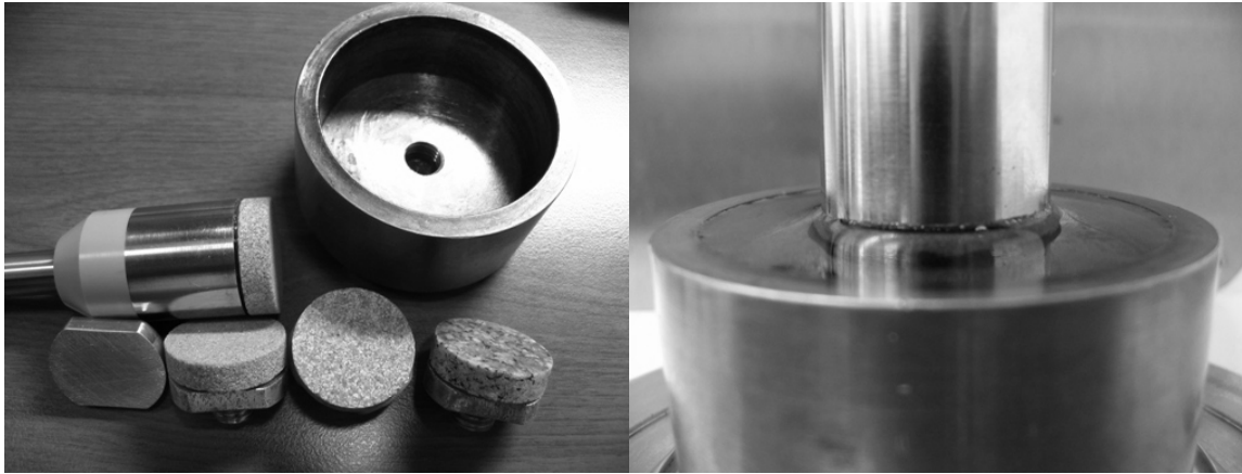
FIGURE 3 DSR testing apparatus: (a) Sample Preparation (b) Wet-Conditioning (22).
