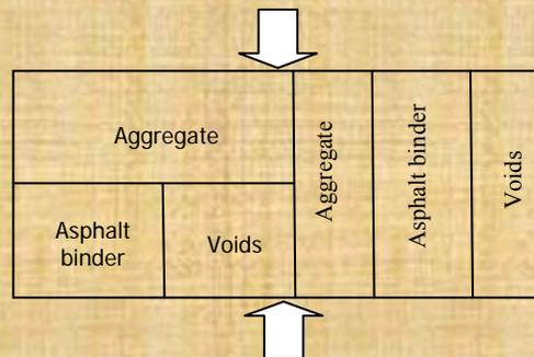
$$E_{mix} = Pc[E_{agg}V_{agg} + E_{binder}V_{binder}] + (1 - Pc) \left[ \frac{V_{agg}}{E_{agg}} + \frac{(1 - V_{agg})^2}{E_{binder}V_{binder}} \right]^{-1}$$
