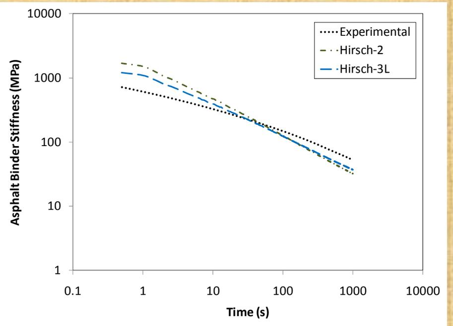
Hirsch model for PG 58-34 M1 mixtures  $T=-24^{\circ}\text{C}$
