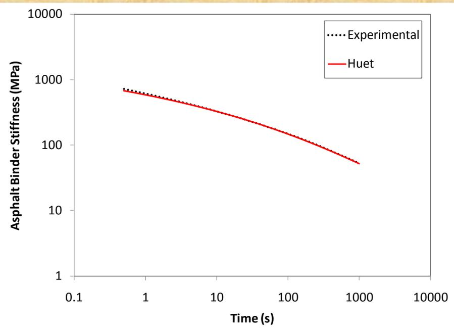
Huet model for PG 58-34 M1 mixtures  $T=-24^{\circ}\text{C}$
