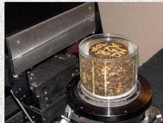
Saturated specimen during X-ray CT scanning
