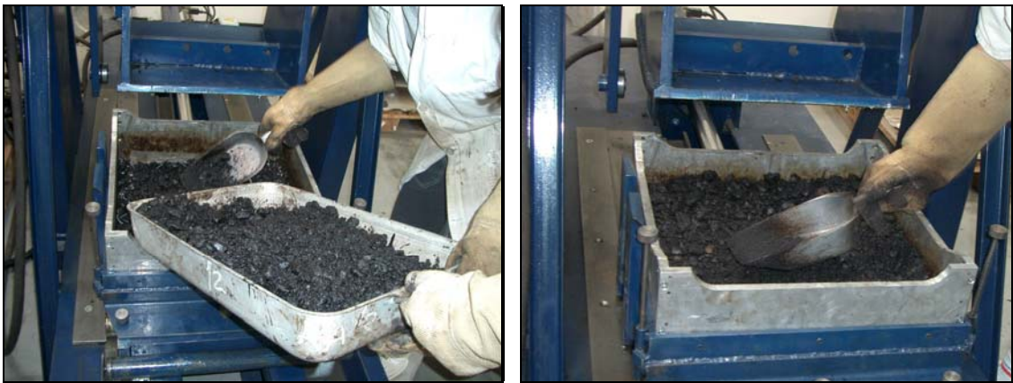
Fig. 4 – Box filling with asphalt concrete
