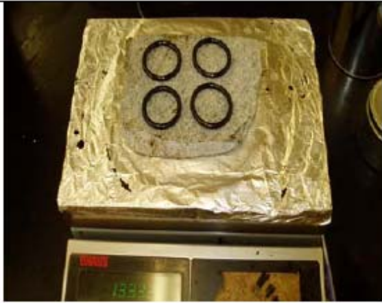
FIGURE 1: Preparation of Aggregate Surface for Emulsion Placement (7)
