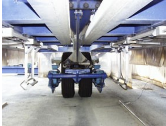
Figure 2.6. Simulated truck tire from accelerated loading facility equipment (From fhwa.dot.gov )
