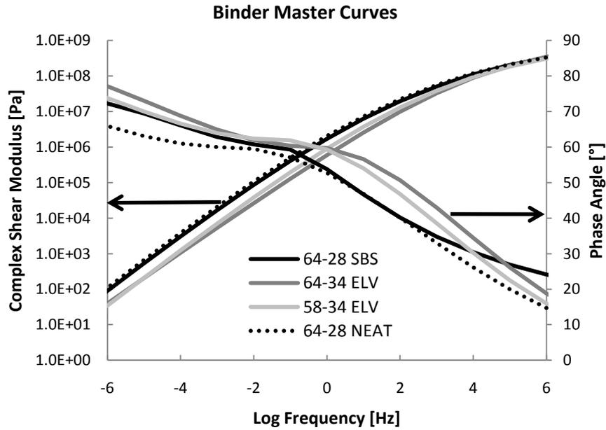
Figure 1. Rheological master curves for the binders used in this study.
