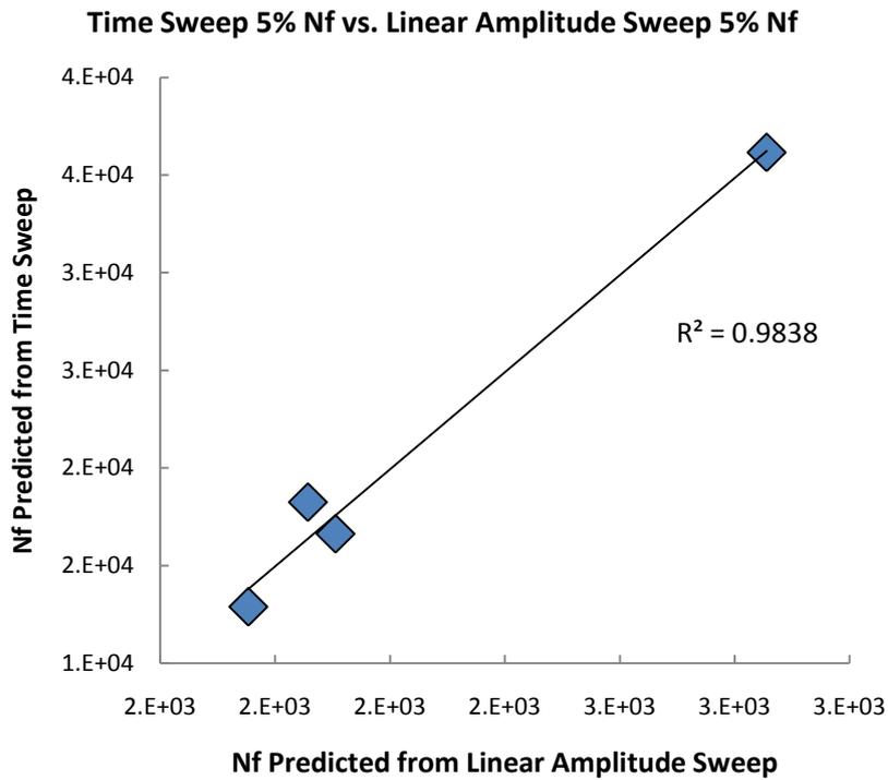
**Figure 8.** Plot of predicted  $N_f$  at 5% applied strain from times sweep and linear amplitude sweep VECD analyses.
