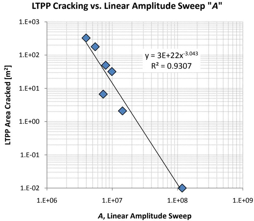
**Figure 11.** Fatigue cracking from LTPP measurements compared to the linear amplitude sweep VECD A parameter.
