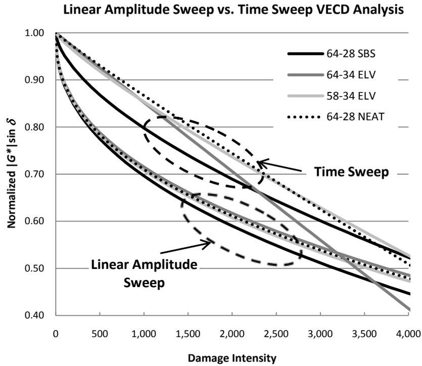
**Figure 6.** Comparison of VECD analysis from linear amplitude sweep & time sweep data.
