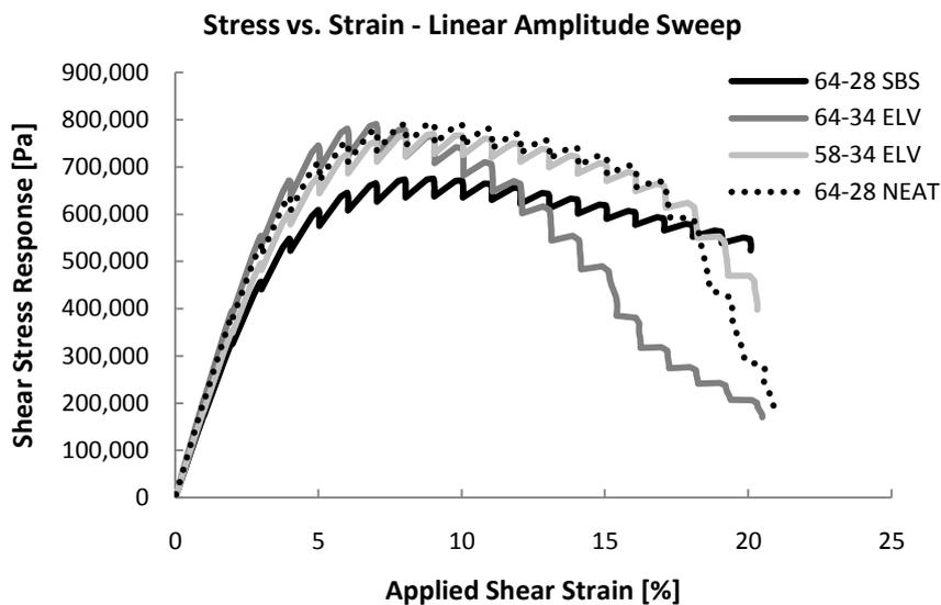
**Figure 4.** Linear amplitude sweep test results for the first replicate testing.
