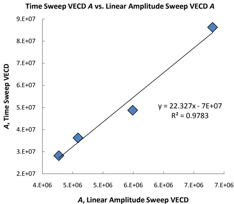
**Figure 9.** Plot of the fatigue law parameter “A” derived from VECD analysis of time sweep versus linear amplitude sweep tests.
