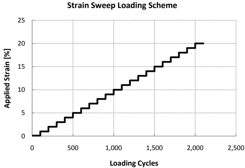
**Figure 2.** Loading scheme for the linear amplitude sweep test employed in this study.
