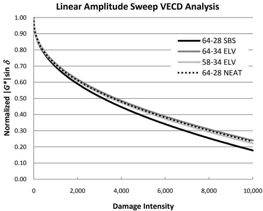
**Figure 5.** Plot of normalized  $|G^*| \sin \delta$  versus damage from linear amplitude sweep testing.
