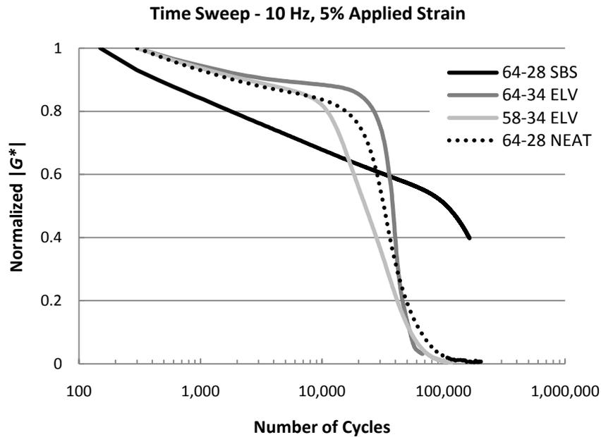
**Figure 3.** Time sweep test results for the first replicate testing at 5.0% applied strain.
