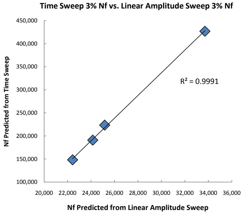
**Figure 7.** Plot of predicted  $N_f$  at 3% applied strain from times sweep and linear amplitude sweep VECD analyses.
