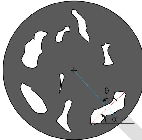
Figure 3. Illustration of orientation angles
