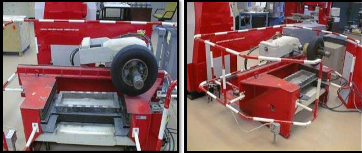
**Figure 3:** LCPC French Roller Apparatus
