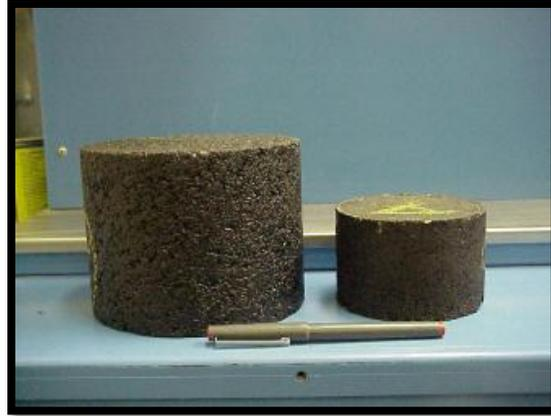
**Figure 9:** *Gyratory specimen shown on left, California Kneading Compactor specimen on right.*
