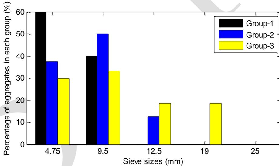
**Figure 6. Example histogram of distribution of different aggregate sizes in each group.**
