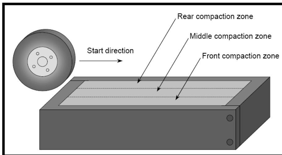
**Figure 4:** Roller Compaction Zones
