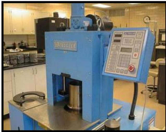
**Figure 7:** *Super PAVE Gyrotory Compactor Apparatus*
