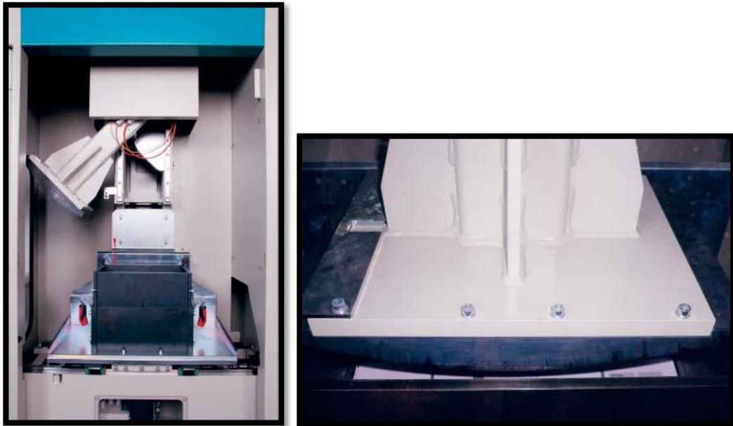
**Figure 5:** *Left: German Sector Compactor before use. Right: Sector compactor during use*
