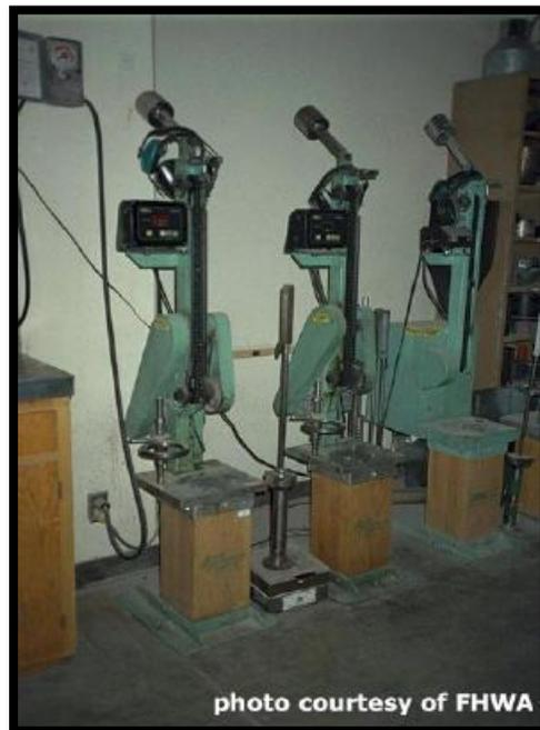
**Figure 1:** *Marshall Impact Hammers*
