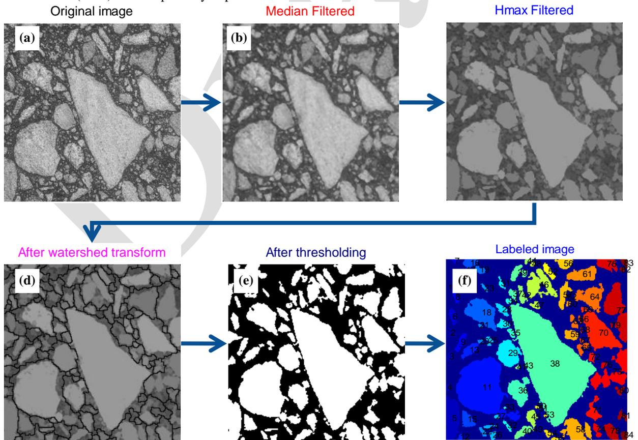
Figure 1. Illustration of steps of image processing filters.
