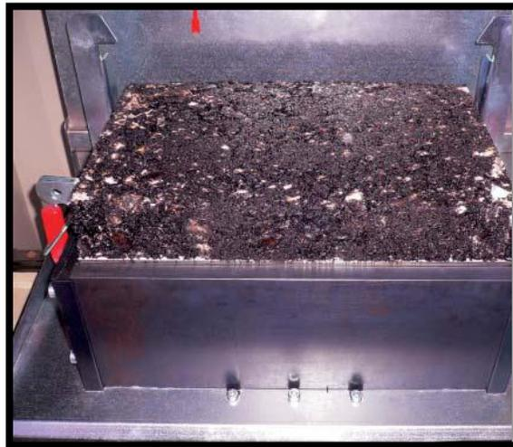
**Figure 6:** Specimen after Compaction
