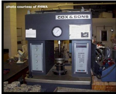
**Figure 2:** California Kneading Compactor
